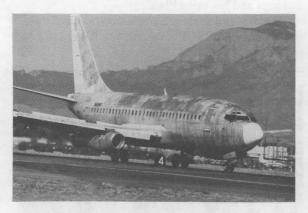
WORSE FOR WEAR — An over-the-hill 737 transport plane lands at Albuquerque. It's now used for research on inspecting aging aircraft.
